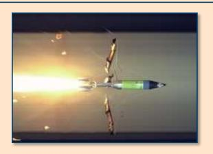
**CENTRIFUGE TESTS:** These tests emulate acceleration forces encountered during test flights and are conducted on safe and armed devices to measure arming devices and electrical parameters.
