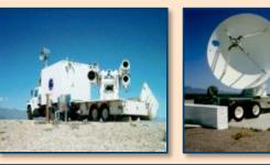
The highly accurate instrumented range allows for target location validation. Tracking devices include high-resolution optics, C and X band radars and Laser radars.
