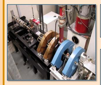
**RAPID RESPONSE LABORATORY (RRL):** The RRL consist of five bench-top stations that enable most types of active semiconductors and components, circuit card assemblies, small system characterization, testing to appropriate INR environments, and post-test analyses.
