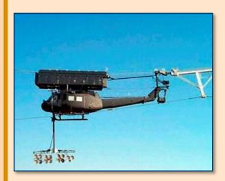
The cable can be adjusted to suspend targets from 100 to 1,000 ft AGL
