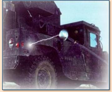
**ELECTROSTATIC DISCHARGE** (ESD) FACILITY: Electrostatic discharge (ESD), or static electricity, can be potentially devastating to sensitive electronics. To ensure that weapon systems are hardened against damage from ESD, we perform both personnel-level (25,000 volts direct current and helicopter-level (350,000 VDC) ESD testing.
