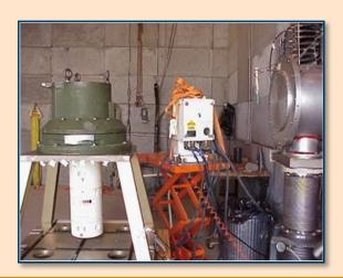
RELATIVISTIC ELECTRON BEAM ACCELERATOR (REBA): The REBA (1.9MeV) and PI 538 (4.2 MeV) is a high-energy, pulse, field emission electron beam or Bremsstrahlung x-ray source. These simulators produce the gamma dose rate environments of a nuclear weapon detonation.
